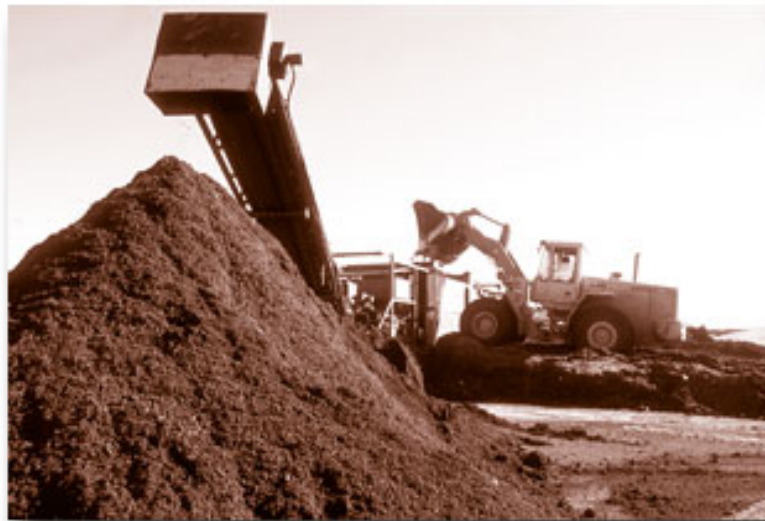
Compost is loaded into a trommel, which screens the material to a fine consistency. As part of its combined operations, TDS sells the decayed organic matter to landscapers and gardeners to fertilize and condition the soil. / Photo by Tommy Hultgren
