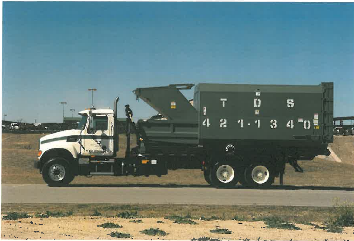
Roll-off truck with self-contained compactor
